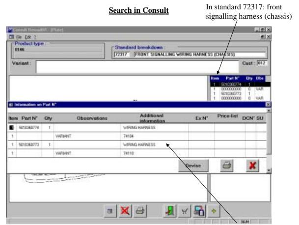
... shows the reference of the harness powering the window washer pump
