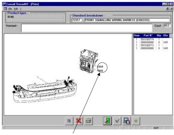
The electrical harness is connected to terminals C812 and C825.
